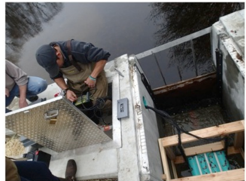
Annual installation of the electronic fish counter at the Rogers Lake Fishway
